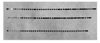
Surprisingly, though, it turned out these thin bridges don't necessarily need repair to be physically scannable or analyzed correctly by the software. As we found out, the scanner runs the roll more smoothly and tightly than we are able to on our manual table - if it doesn't present issues for us, then it rarely presents issues for the scanning operation.
