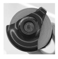
Endcap damage is when the part of the flange outside the core has portions broken off. With care and practice, the scanner operators can scan rolls with a large amount of the endcap missing, but there is some risk that the paper edge may catch on the remaining part of the endcap or be difficult to keep aligned.
